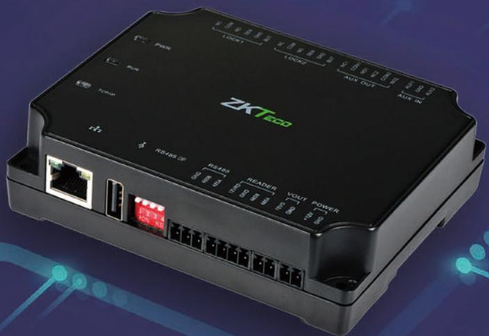
C2-260 is an IP-based two doors mini control panel. It supports TCP/IP communication through LAN or WAN network, and RS485 communication which allows extension to RS485 devices like DM10, AUX485, WR485. The series is a perfect match for the web-based software ZKBioAccess to provide RFID Security solution. C2-260 can control two doors by default. It can extend to 8 DM10s at most that it can support up to 10 doors.
